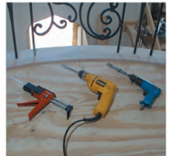
TOOLS USED: Standard Electric Drill, Air Hammer/Chisel, Epoxy Gun
